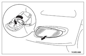
2. Slide the light unit outward to remove it. Turn the light socket counterclockwise and pull it out.
